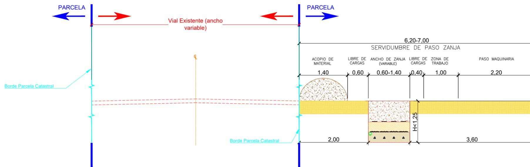
ZANJA RSMT 18-30 KV PARALELA A VIAL EXISTENTE
