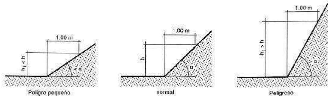
***Fig. 1: Talud natural de  $\alpha'$***
