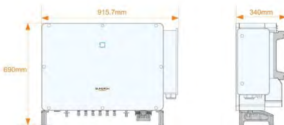
Figure 2-3 Dimensions of the Inverter (in mm)
