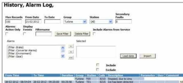
Figure 3 - Presentation of alarms related to the ice detection system in Web WPS SCADA
